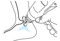
**17** Use the Pivot Punch tool (available for purchase) to quickly and accurately create your mounting holes in the AFO. If you don't have a Pivot Punch tool, use a 13/64" or a 5mm bit to drill mounting holes into the dimples, created by the Indexed Hole, at the top and bottom of the hinge plate cavities.
